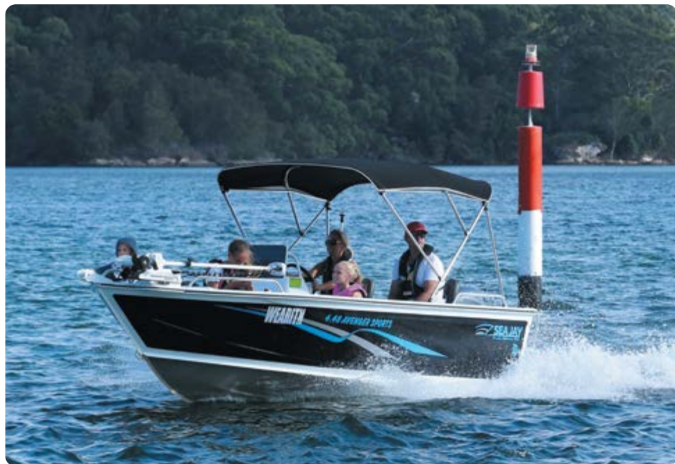
Powerboat passing a port mark (red) while heading downstream.
